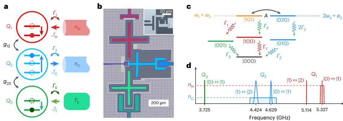
**Fig. 1 | Quantum-absorption-refrigerator scheme and level diagram.**
